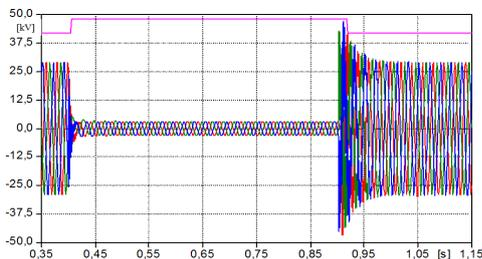
Fig. 13. Line to line MV voltages and voltage dip detection signal (magenta)
