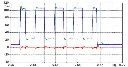
Fig. 8. Reactive power: load (blue), grid (red), inverter (green)
