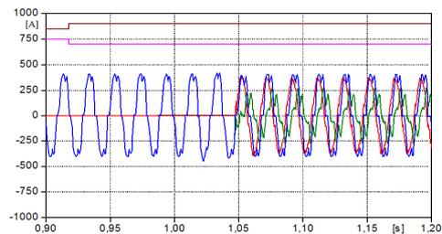
Fig. 16. Phase "c" currents at the end of island operation: grid (red), load (blue), inverter (green); voltage dip detection signal (magenta); static switch trip (brown)
