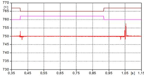
Fig. 17. DC voltage during the island operation; voltage dip detection signal (magenta); static switch trip (brown)
