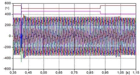
Fig. 14. Line voltages in island at the beginning of the voltage dip, for non-linear load; voltage dip detection signal (magenta); static switch trip (brown)
