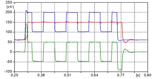
Fig. 7. Active power: load (blue), grid (red), inverter (green)
