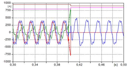
Fig. 15. Phase "c" currents at the beginning of island operation: grid (red), load (blue), inverter (green); voltage dip detection signal (magenta); static switch trip (brown)
