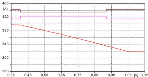
Fig. 18. SMES current trend (red) during the island operation; voltage dip detection signal (magenta); static switch trip (brown)
