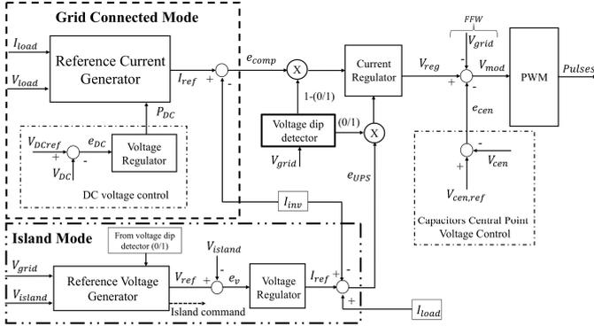
Fig. 5. General control system blocks scheme
