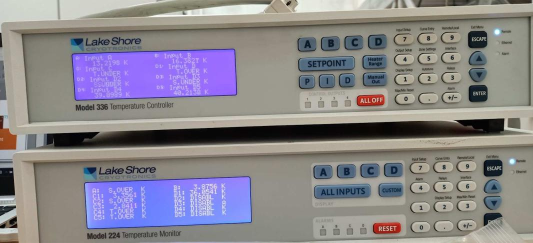
**3.9 K reached on the coil in no load condition**
