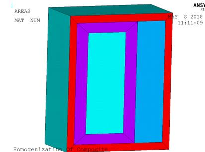
Thermal transient on a 15° sector made of 4x4 strand is calculated
