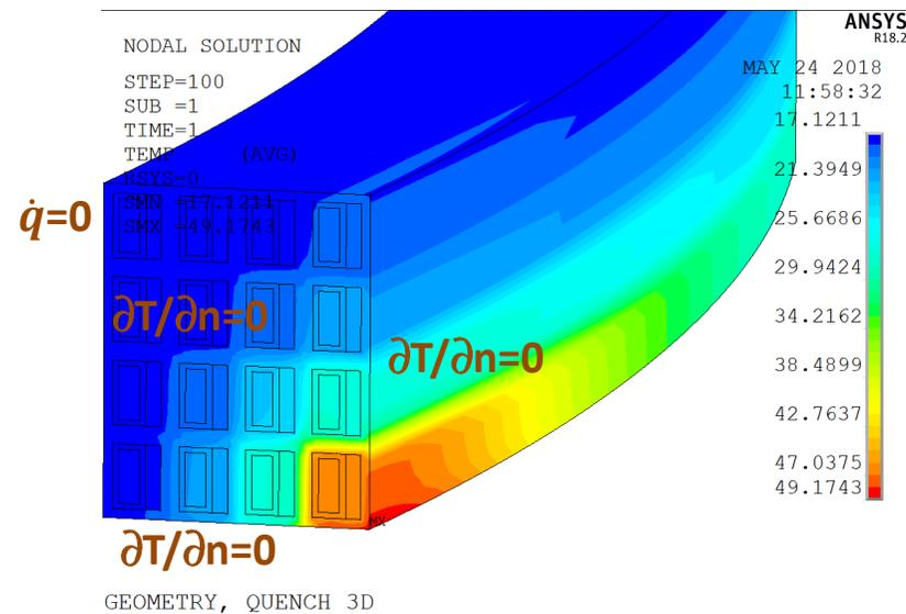
A max temperature of 108 K is reached in the coil
